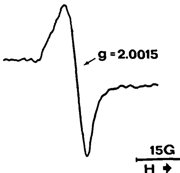
Figure 1. A typical, room temperature, ESR spectrum of freshly ground quartz particles.
