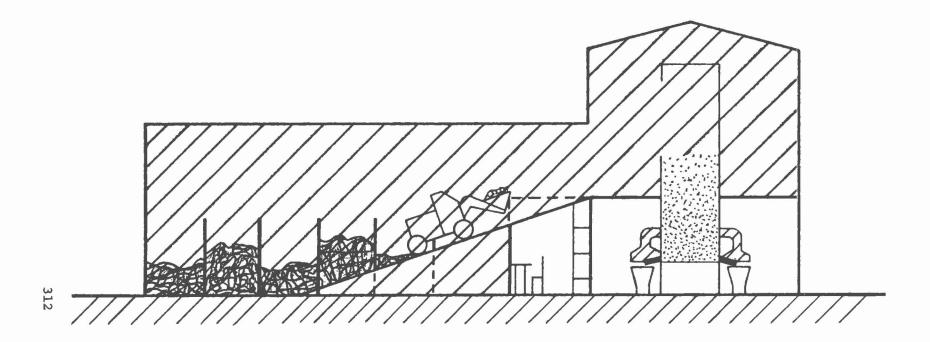
Figure 1. Clean and dirty rooms around the SB-furnace (in the tall building at right).
