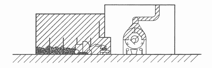
Figure 1. Clean and dirty rooms around the SB-furnace (in the tall building at right). The hatched areas indicate dirty rooms for reception and storage of raw material and for charging the furnace. Only the machine cabin is a "workroom". The tapping bay around the base of the furnace and the adjacent control room are controlled to low lead-in-air values.
