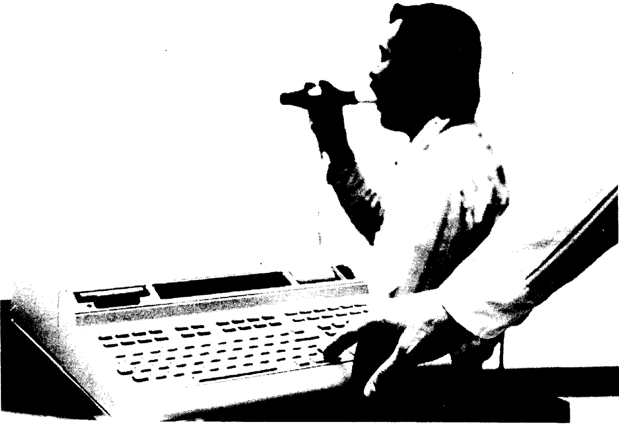
Figure 6-7. Hewlett-Packard 47804A, a flow measuring spirometer. (Courtesy of Hewlett-Packard, Andover, Massachusetts).
