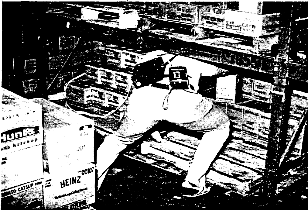
Figure 3.3: An Example of a Three-Slot Configuration (Top) and Body Posture Used to Pick Up a Load from the Bottom Slot (Bottom)
