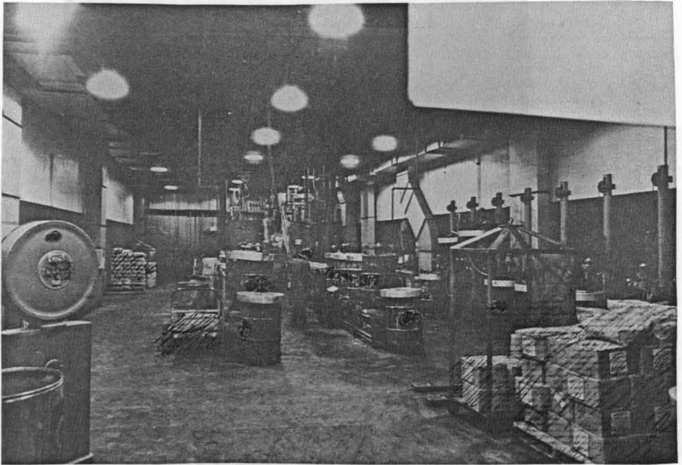
Figure 7-4. Cement house showing cowl mixers to right, and agitators and drum racks in center. Also, note palletted materials.
