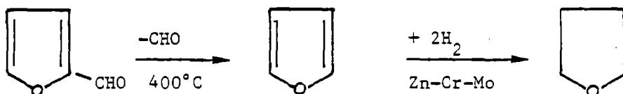
The assumed yield from this process is 75% [4]. Furfural is obtained from a variety of raw materials that occur as waste products from food processing, including oat hulls. Quaker Oats operates the only furfural based THF plant, which is located in Memphis, Tennessee.
