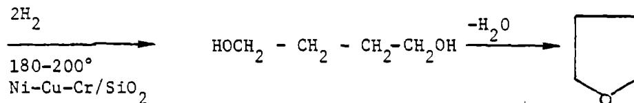
The final step proceeds at 110-120°C in the presence of phosphoric and sulfuric acid. An alternate method is to carry out the dehydration of 1,4-butanediol in a high pressure reactor (300°C, 100 bar) in the presence of acid. The selectivity to THF in this process is greater than 95% [6].
