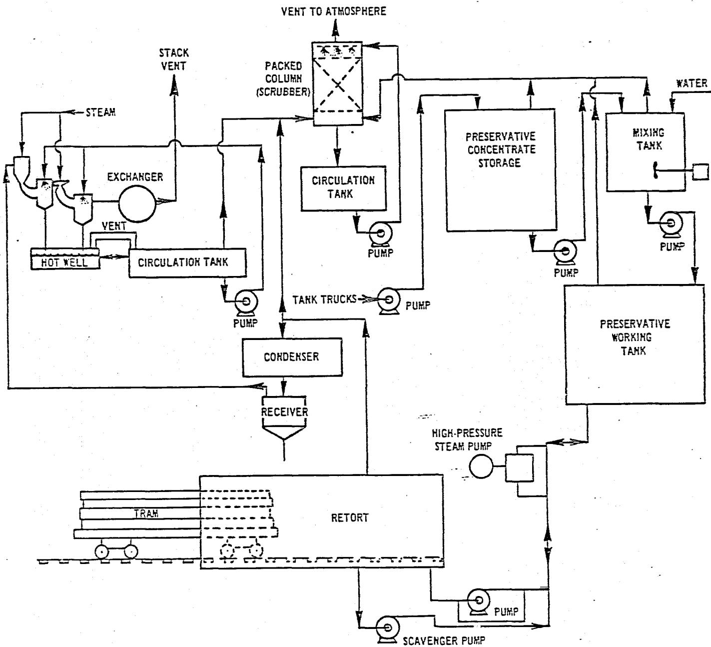
Figure 3-1 Flow Diagram for the Full-Cell Pressure Process
