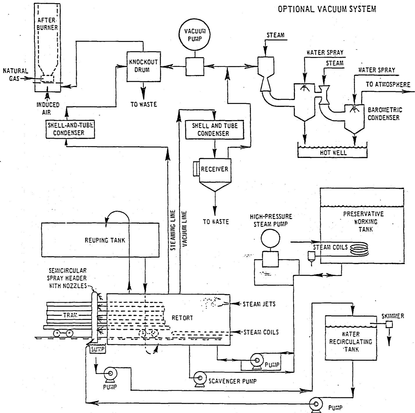
Figure 3-2 Flow Diagram for the Empty-Cell Pressure Process
