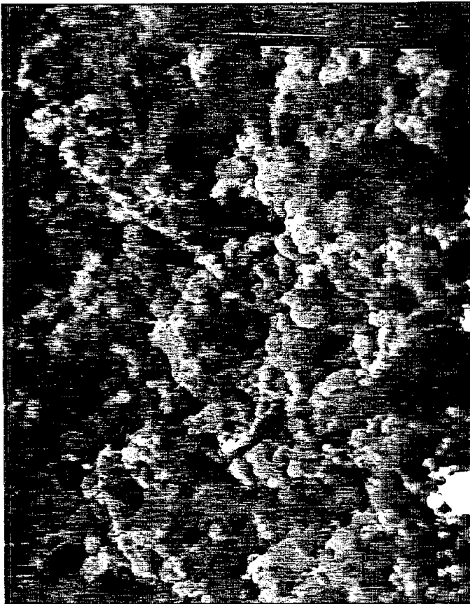
Figure 3C. Mild steel, stick fumes, AAWP, 6000x. Figure 3D. Stainless steel, stick fumes (6000x)
