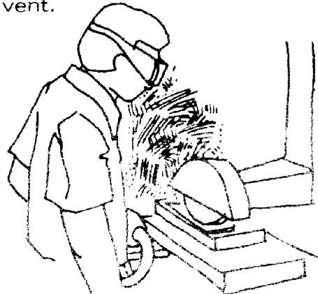
... Air from fans or other sources near you are blowing dust and mists away from the exhaust vent and into your face.
