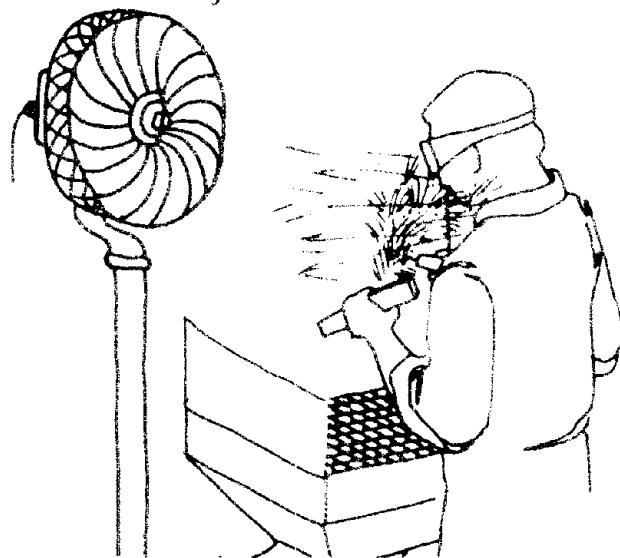
... Contaminated air is being recirculated back into the work area.
