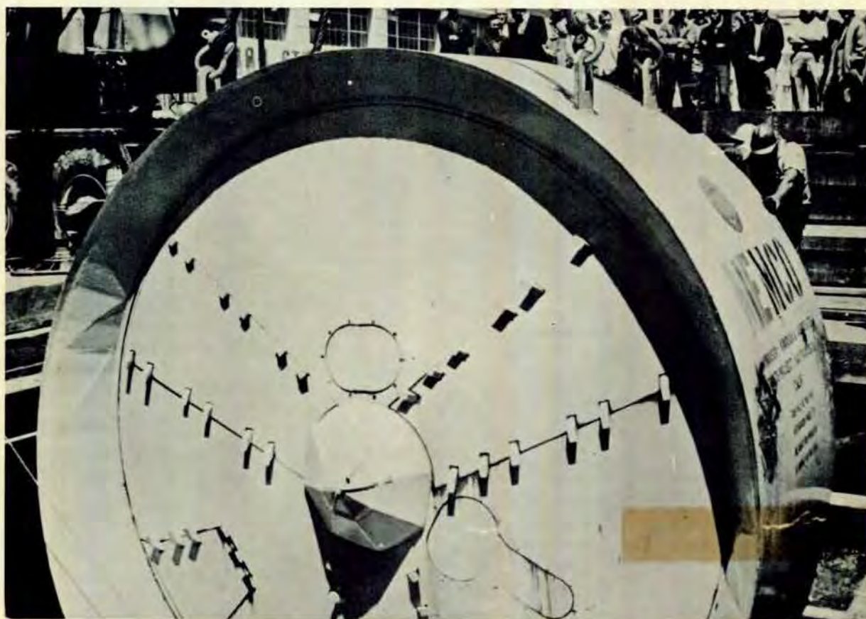
FIG. 2. Cutting wheel of soft-ground tunneling machine used in BART project.
