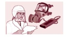
easier to breathe through and they need a fully charged battery to work properly. They use the same filters as gas masks, so you need to know what the hazard is, and how much of it is in the air.
