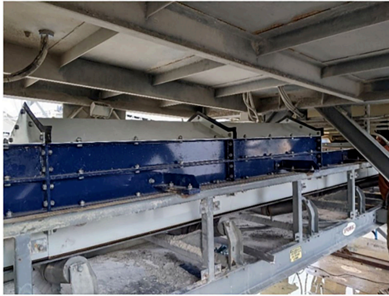
Fig. 1. Passive dust reduction system tailored to the #15 conveyor at CPM, based on Benetech®'s MaxZone® technology. The system comprises shrouds in sections with baffles at each junction, and a patented belt sealing interface with “XN liners” and dual-rubber adjustable seal
