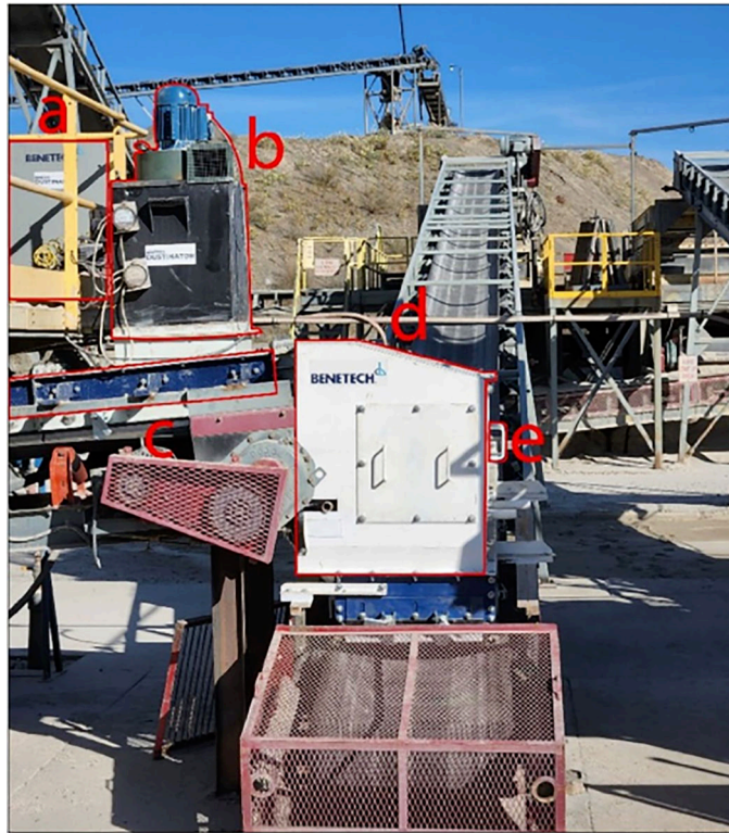
Fig. 7. Crusher/conveyor system at the CPM site, after installation of the dust control system: (a) MiniPak cabinet, (b) Dustinator, (c) shrouding/belt sealing system, (d) transfer point enclosure, (e) spray bar (at exit)
