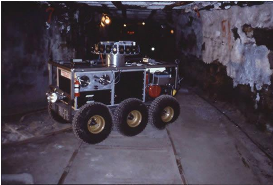
Figure 8 Terregator robot developed by CMU in partnership with NIOSH for mine mapping.
