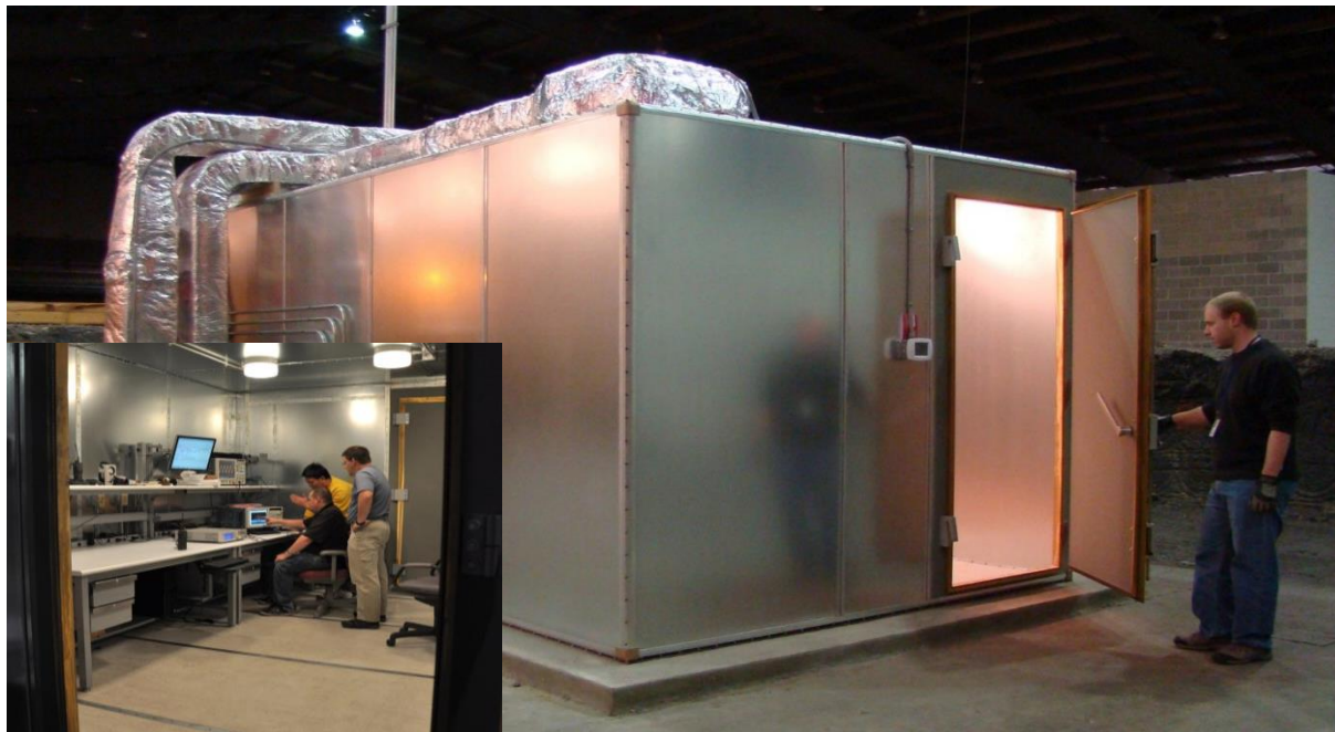
Figure 16. Exterior and cutaway of interior of radio frequency (RF) shielded lab.
