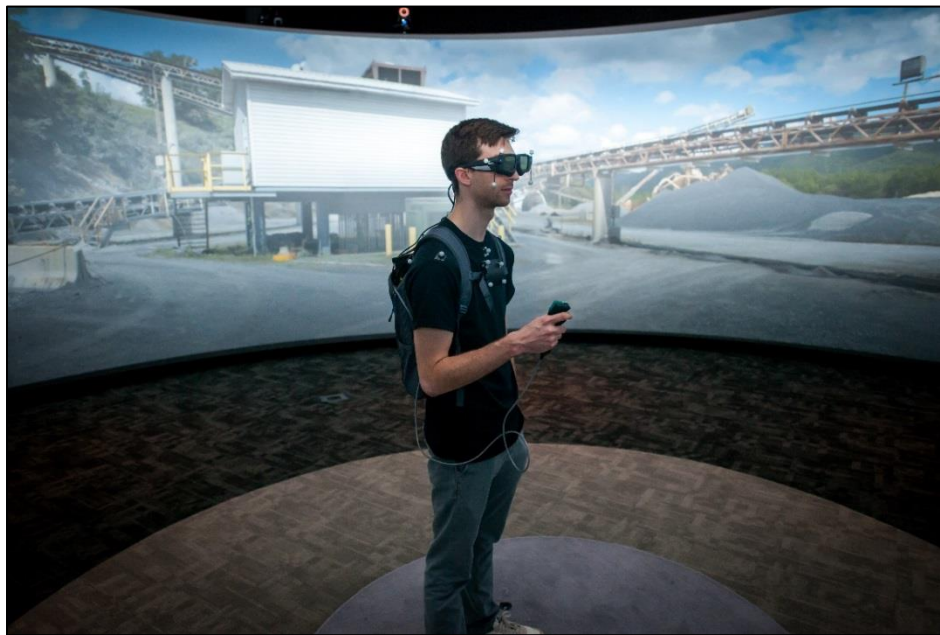
Figure 15. Eye tracking of panoramic mine scenes in the VISIlab laboratory.
