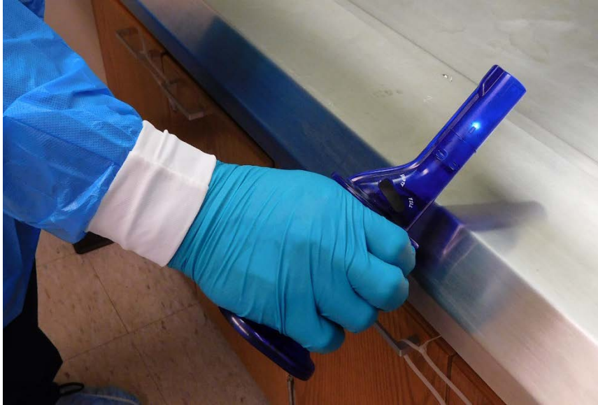
Figure 4. Example of a qualitative smoke test with Wizard Stick Smoke Generator (Photo Credit: NIOSH)
