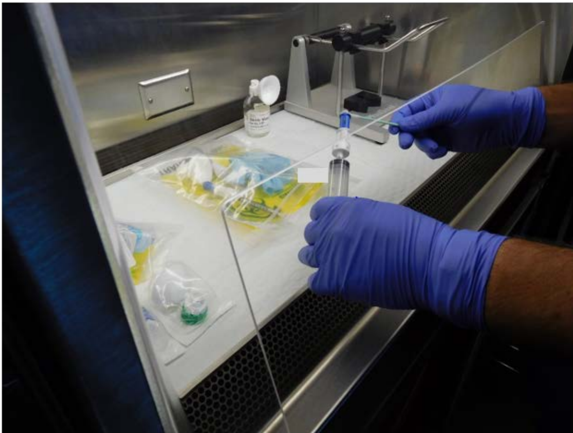
Figure 27. Intentional “Hot” wipe sample collected from carboplatin syringe with CSTD adapter. Also shown: PhaSeal vial adapter and adsorbent pad. (Photo Credit: NIOSH)
