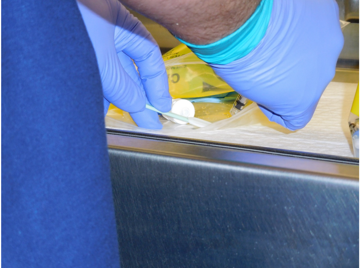
Figure 30. Intentional “hot” wipe sample collected from within a vincristine transport bag (Photo Credit: NIOSH)
