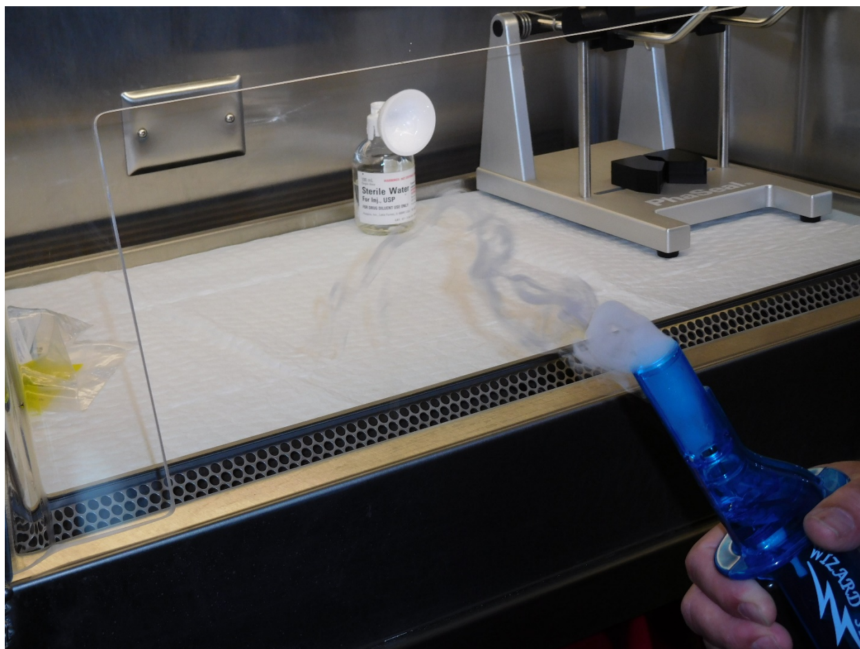
Figure 8. Qualitative smoke test with Wizard Stick Smoke Generator (Photo Credit: NIOSH)
