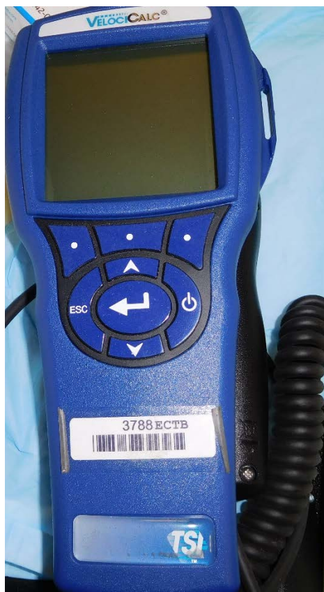
Figure 4. TSI® VelociCalc™ Plus Model 9565-P thermal anemometer (Photo Credit: NIOSH)
