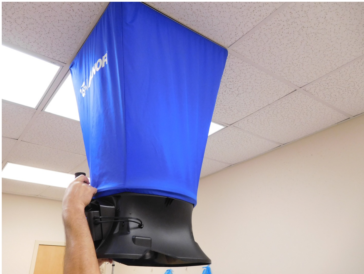
Figure 6. TSI Accubalance® Plus Air Capture Hood (Photo Credit: NIOSH)
