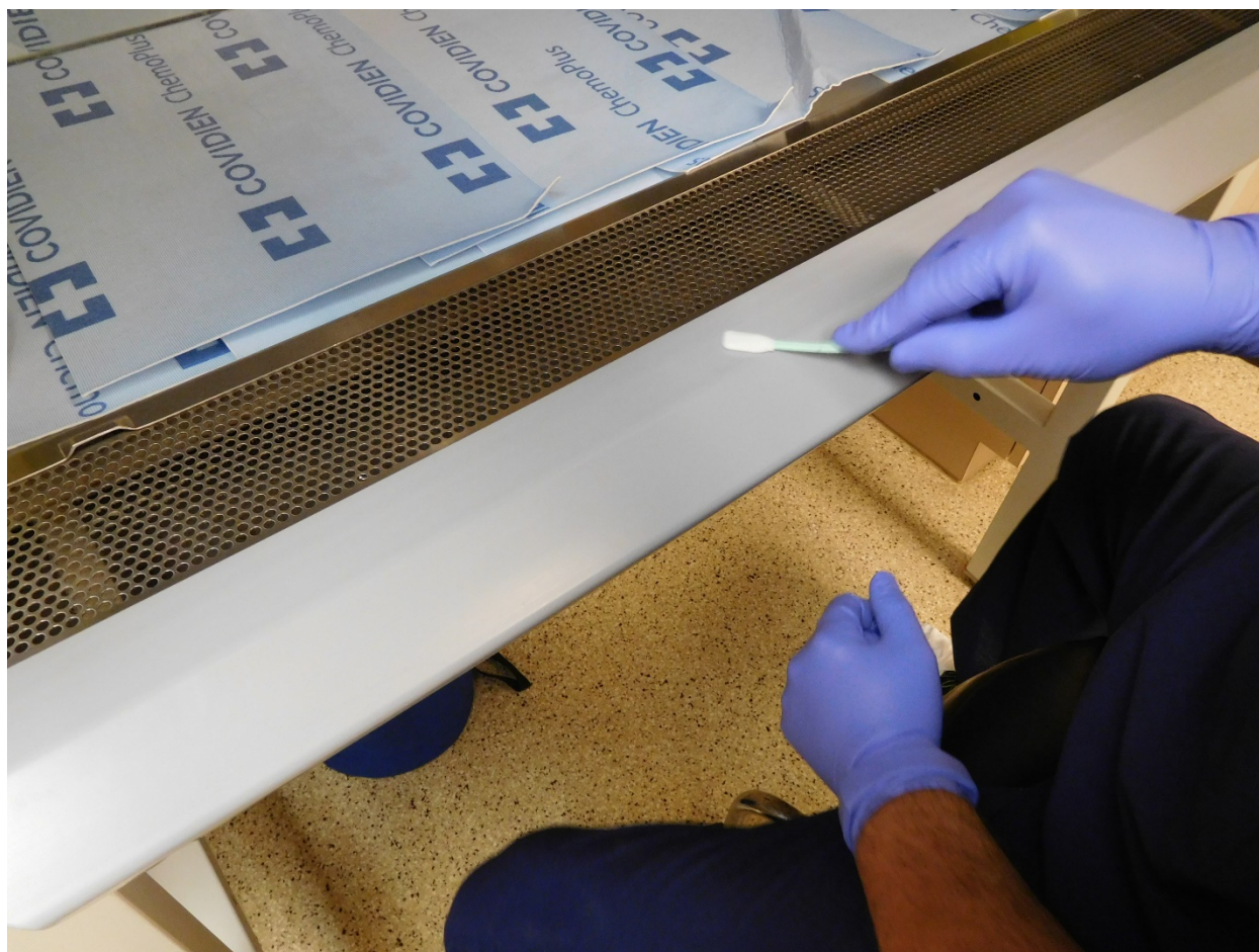
Figure 9. Surface wipe sample collected on BSC's airfoil and lip (Photo Credit: NIOSH)
