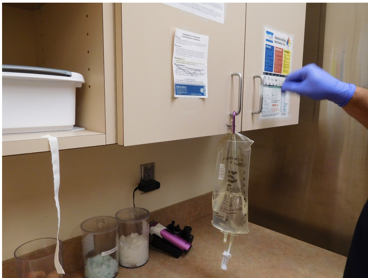
Figure 12. Surface wipe sample collected from storage cabinet handle (Photo Credit: NIOSH)
