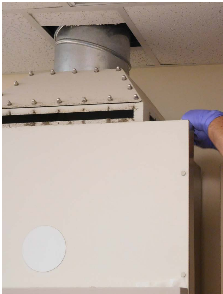
Figure 10. Surface wipe sample collected downstream of BSC's HEPA filter (Photo Credit: NIOSH)
