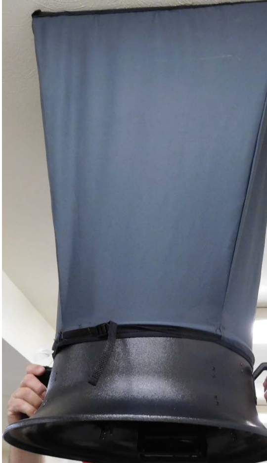
Figure 9. Example of a TSI Accubalance® Plus Air Capture Hood (Photo Credit: NIOSH)
