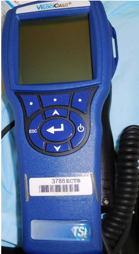
Figure 7. Example of a TSI® VelociCalc™ Plus Model 9565-P thermal anemometer (Photo Credit: NIOSH)
