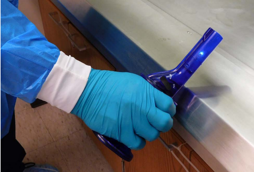
Figure 8. Example of a qualitative smoke test with Wizard Stick Smoke Generator (Photo Credit: NIOSH)
