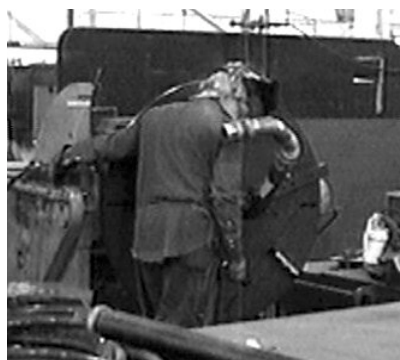
Figure 22. Welder Inspecting Weld Bead, Piece Position
