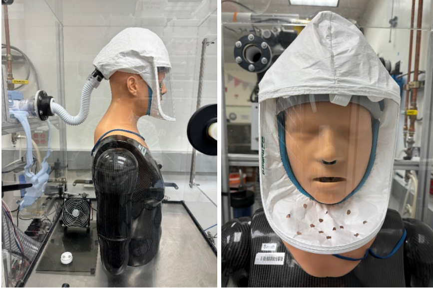
Figure S2: Bullard Salus HC-M PAPR blower and standard facepiece with vent holes below the chin (catalog # 20LF2L, medium/large, NIOSH TC-21C-1235). The PAPR blower was placed outside the test chamber. The PAPR hose ran from the blower outside through an opening and to the PAPR facepiece.
