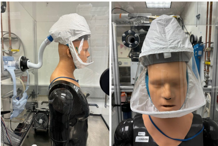
Figure S3: Bullard Salus HC-M PAPR blower and facepiece with a HEPA filtration panel below the chin instead of vent holes (catalog # 20LFMHE, small/medium, NIOSH TC-21C-1237). The small/medium size facepiece was used rather than the medium/large because the small/medium formed a better face seal.
