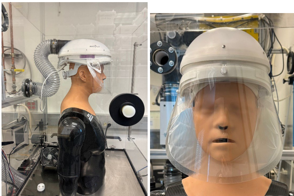
Figure S6: Syntech International Maxair PAPR helmet and face cuff (catalog # 2365-02ML, medium/large). The PAPR ensemble included a new model of filter (2181XP) for which NIOSH approval is pending. Because the Maxair blower is in the helmet rather than worn on a belt, a hole was cut in the plastic cover cap, a custom adaptor was glued to the hole, and the adaptor was connected to a 3" (7.6 cm) hose leading outside the chamber. The perimeter of the helmet cover cap was blocked so that the blower pulled air from outside the chamber through the hose and into the PAPR rather than through the perimeter vent.
