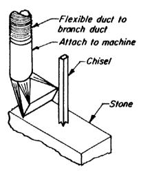
Abrasive blasting to be done in a room or cabinet; 500 fpm at all openings. See "Abrasive Blasting," VS-101
