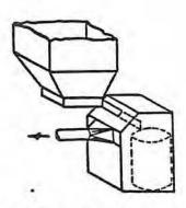
Q=150 cfm/sq ft open face area Duct velocity = 3500 fpm minimum Entry loss = 0.25 VP for 45° toper
