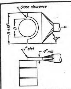
Q = 100 cfm/sq ft barrel top min Duct velocity = 3500 minimum Entry loss = 0.25 VP + 1.78 slot VP Manual loading.
