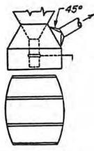
Q = 300-400 cfm Duct velocity = 3500 fpm min Entry loss = 0.25 VP
