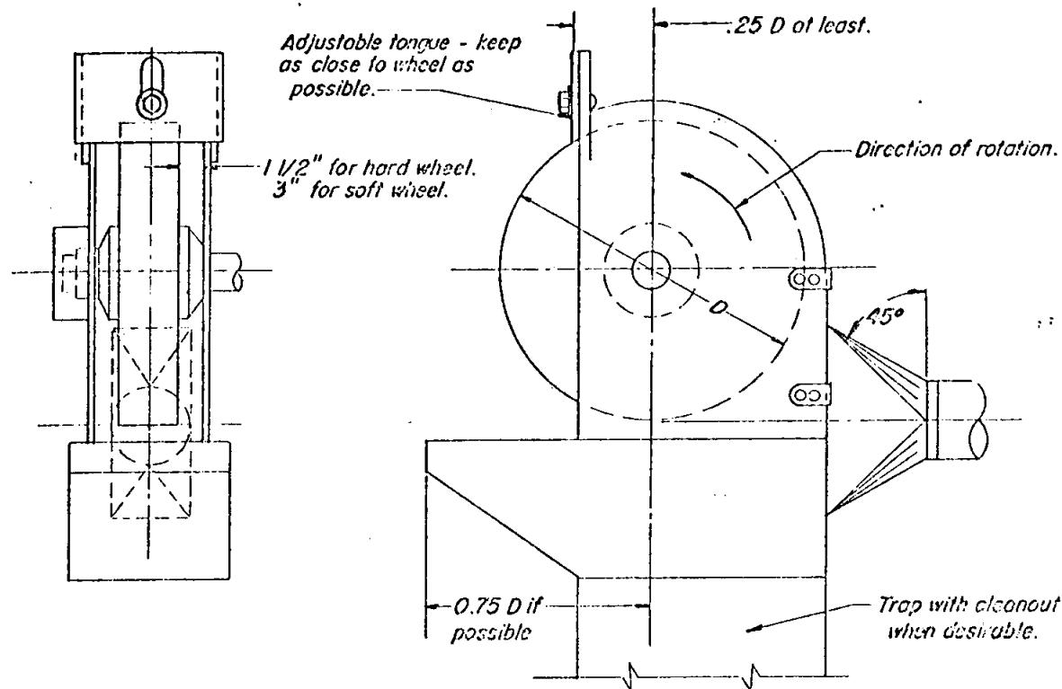
Minimum duct velocity: 4500 fpm branch.
