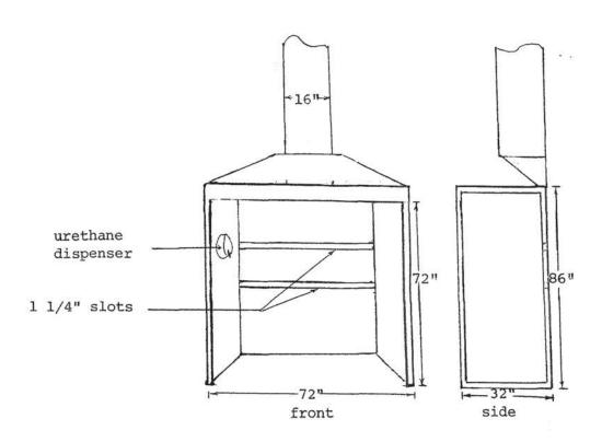
Figure 1 Diagram of the ventilation booth on the Corvette Assembly Line.
