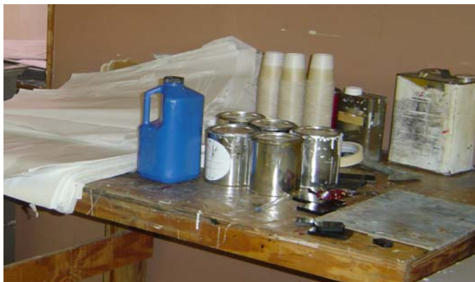
Figure 1. Plastic containers used for lacquer thinner were not approved containers for flammable liquids.
