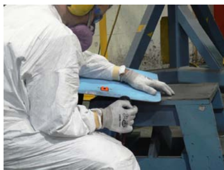
Figure 1. Employee using a handheld grinder to grind composite material.
