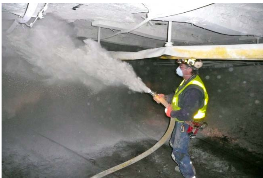
Figure 2. Spraying rock dust onto the surfaces inside the coal mine.
