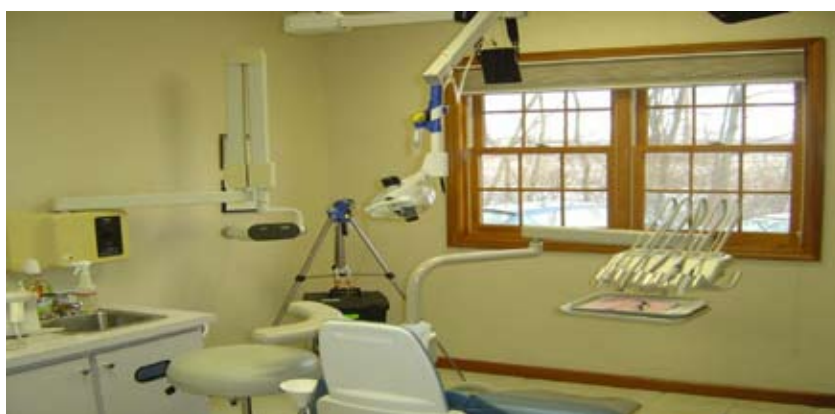
Figure 3. Two-stage bioaerosol sampler mounted on a tripod in the corner of an exam room at Dental Practice A. (Note: Additional sampler on support arm of exam light above dental chair.)
