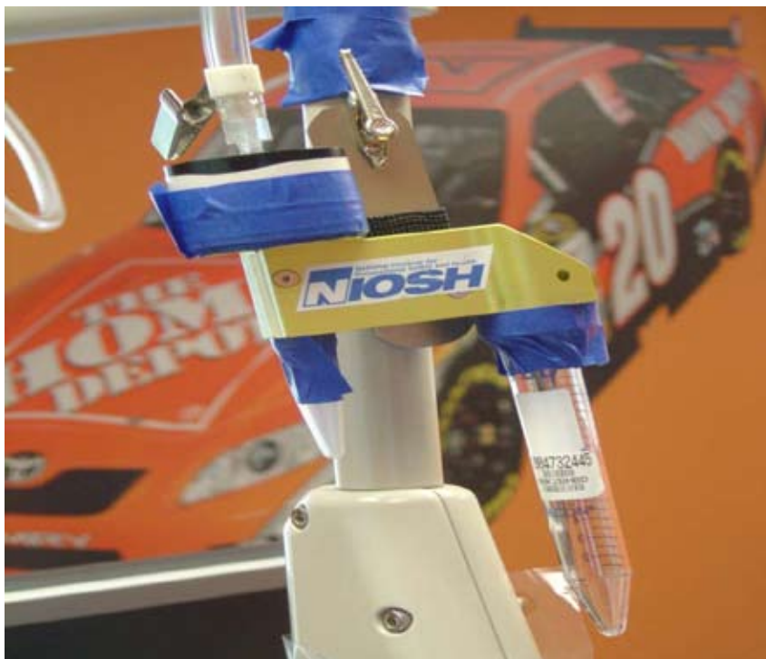
Figure 1. Close-up of NIOSH two-stage cyclone bioaerosol sampler mounted on dental light fixture.
