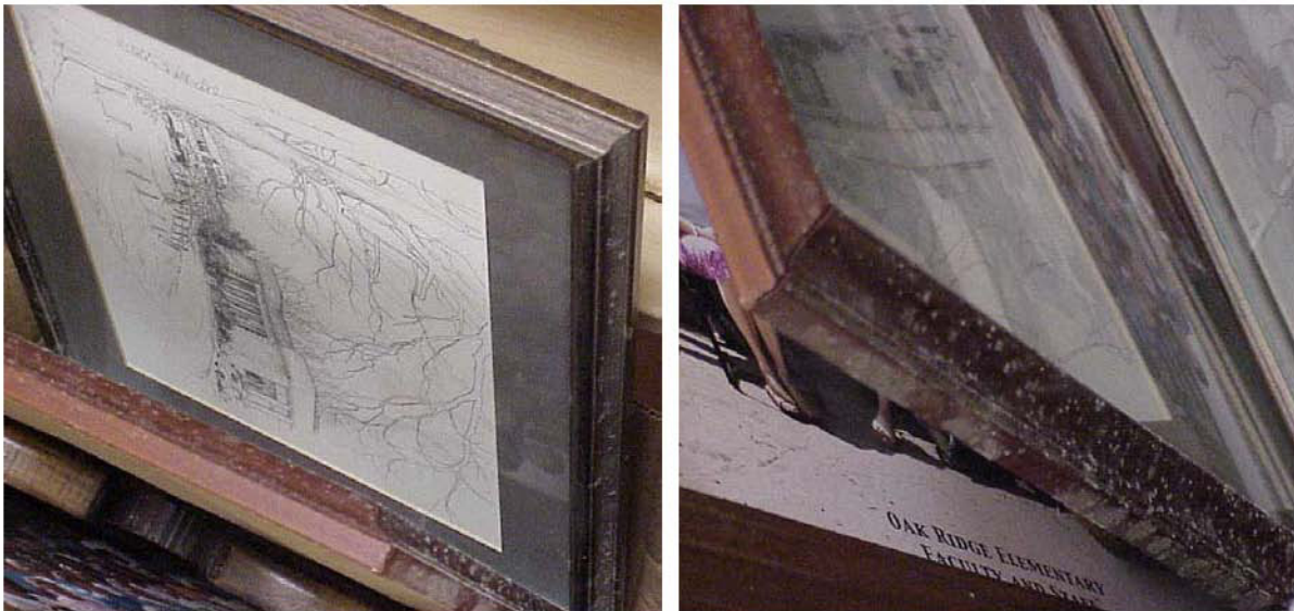
Figure 4. Visible mold on picture frames in the storage room (room 111), August 10, 2005 (courtesy of building occupant)
