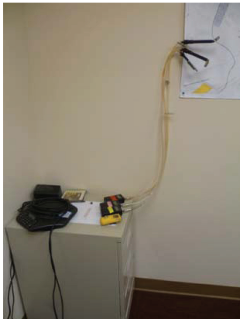
Figure 1. The air sampler inlets were positioned 5 feet above the floor to measure hydrogen sulfide, formaldehyde, and VOCs.
