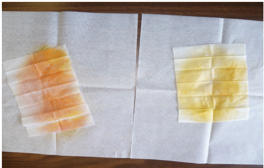
Figure 7. The left wipe, taken from a student who had just returned from the shooting range and had not yet washed hands, is positive for lead. The right wipe, taken after the student had washed hands, is negative for lead.
