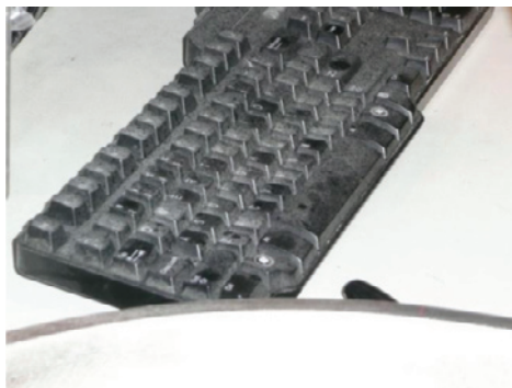
Figure 16. White dust covering a computer keyboard at the workstation of an employee who did offline replenishment of Baker cells.
