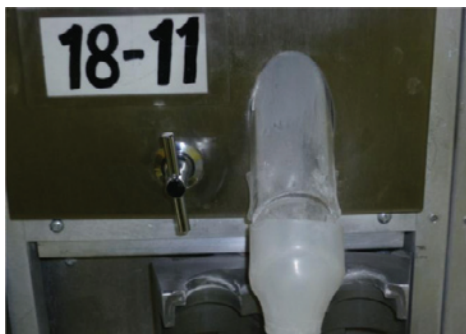
Figure 2. Baker machine nozzle where pharmaceuticals were dispensed into prescription bottles.
