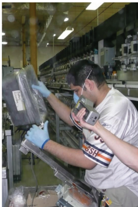
Figure 5. Using a real-time particle meter to measure particle counts near the PBZ of an employee cleaning a Baker cell.
