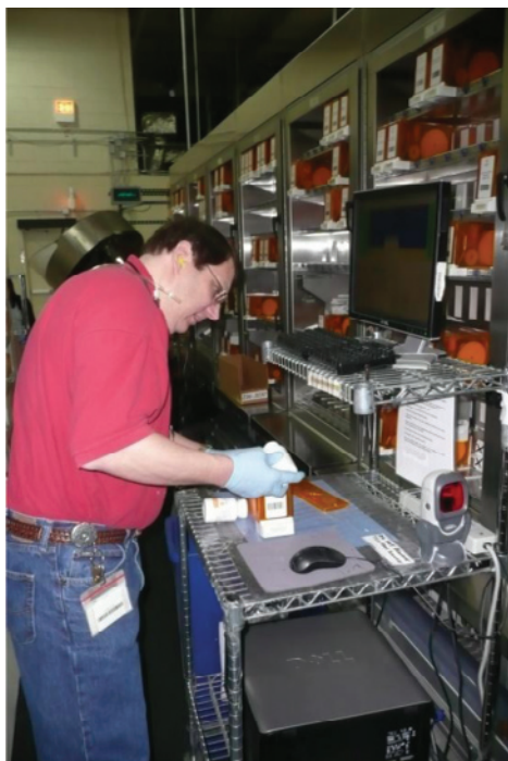
Figure 4. Employee replenishing an Optifill canister with the Optifill machine in the background.
