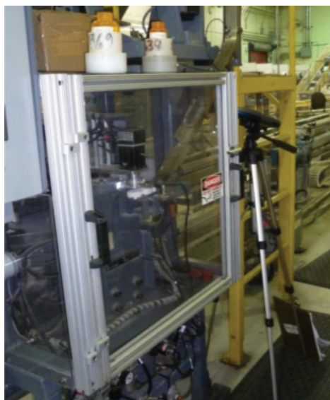
Figure 20. The capper unit enclosure.
