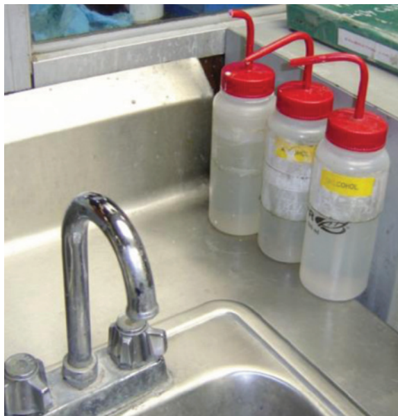
Figure 8. Labels on containers of alcohol in a quality control lab did not include hazard information to warn users of possible adverse health effects from the product.
