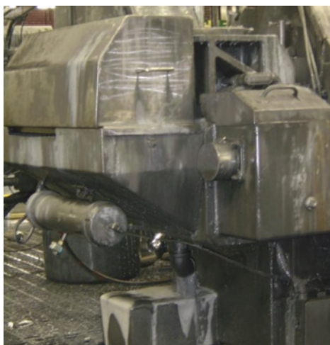
Figure 3. MWF overflowing from an ironer.
