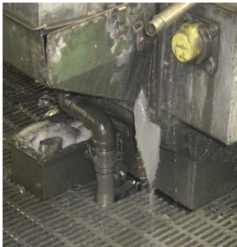
Figure 2. Leaking MWF at an ironer.
