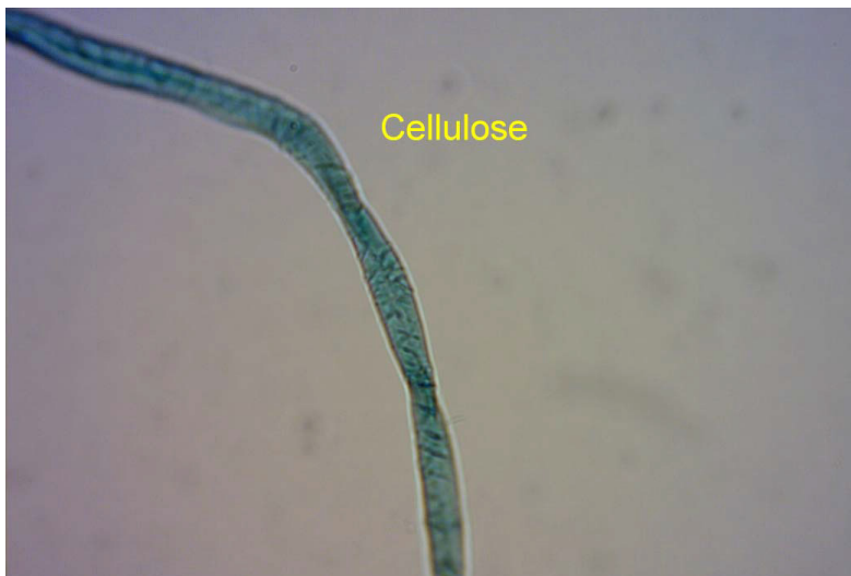
Figure C10. Photomicrograph showing cellulose from sleeve.
