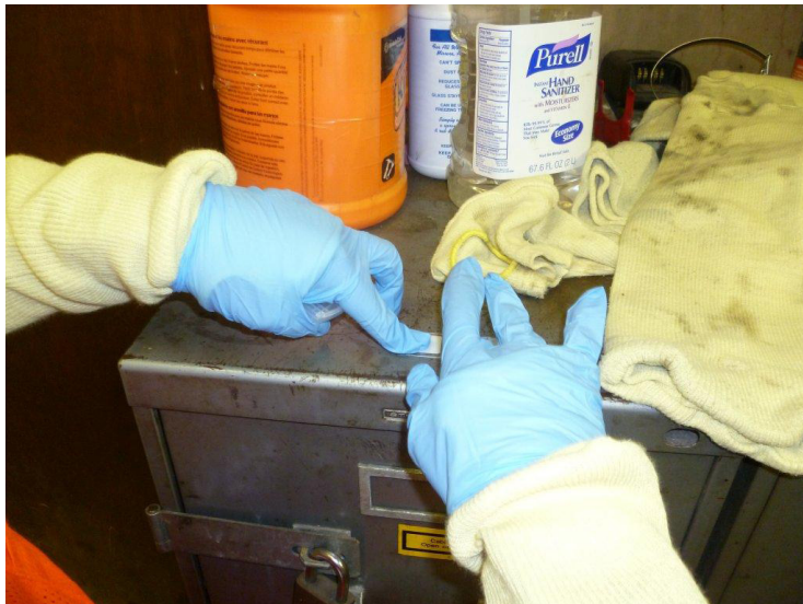
Figure A1. Tape sampling of a surface where cut-resistant sleeves were stored.
