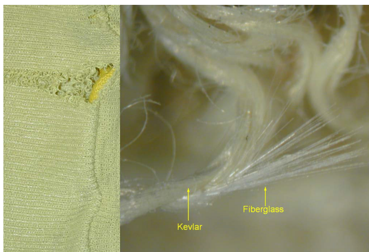
Figure C6. Photomicrographs showing tear in sleeve. RIGHT: Showing broken fiberglass bundles in tear at 15X.
