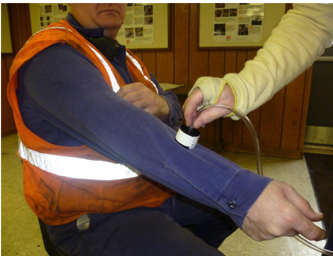
Figure A4. Vacuum sampling on an employee's uniform sleeve after removing the cut-resistant sleeve.
