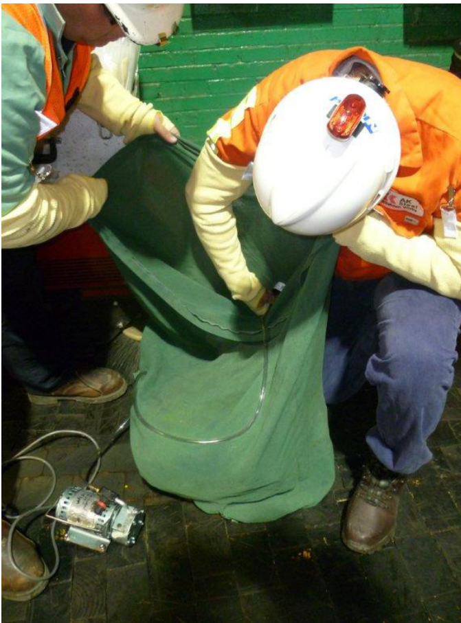
Figure A3. Vacuum sampling of the surface of a bag that stored new cut-resistant sleeves.
