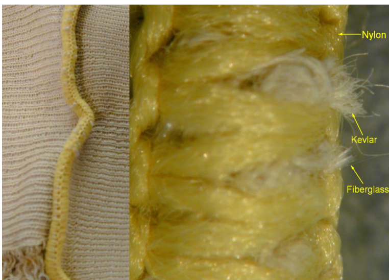
Figure C4. Photomicrographs showing a laundered wrist seam. RIGHT: Showing Kevlar and broken fiberglass bundles coming through nylon seam at 20X.
