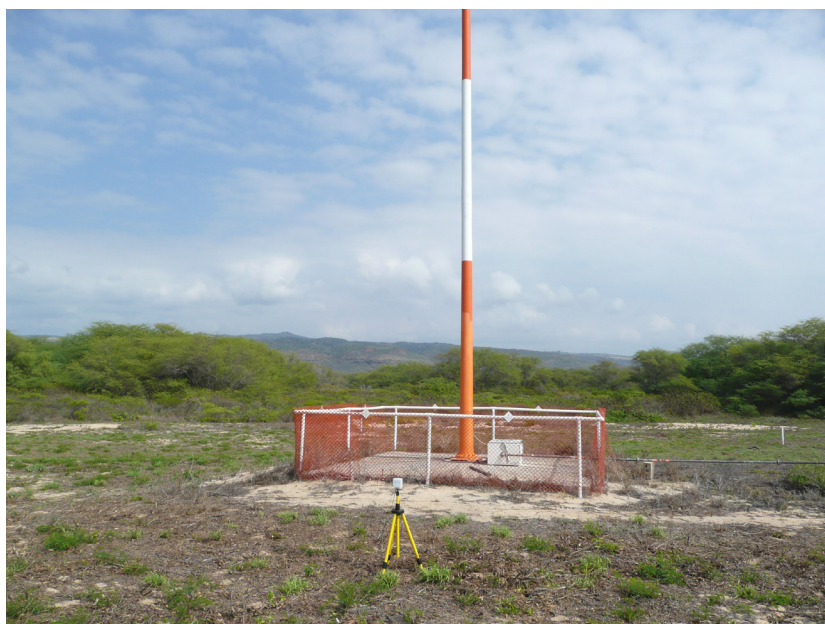
Figure 2. A Narda RF field analyzer measuring RF electric and magnetic fields near the primary 2.5-MHz antenna. Photo by NIOSH.
