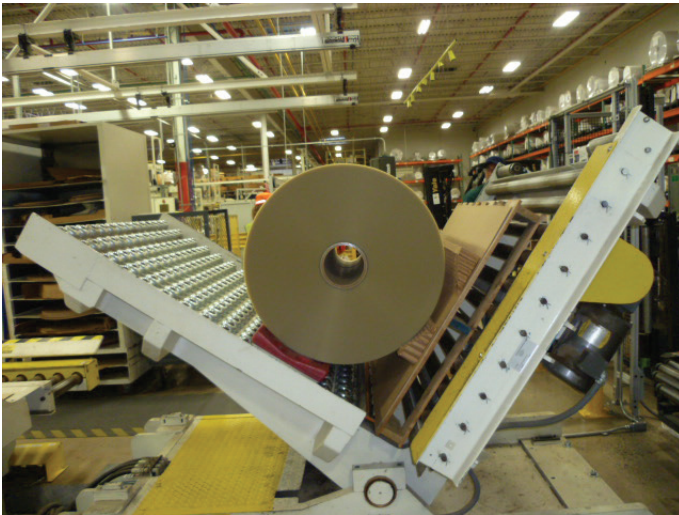
Figure 1. The upender transferring a roll of labels from a horizontal conveyor (left side of the picture) onto a pallet for shipping (right side of the picture). Photo by NIOSH.
