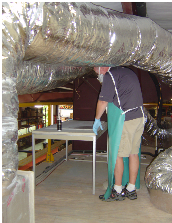
Figure 2. Applying laser marking spray to parts. Photo by NIOSH.
