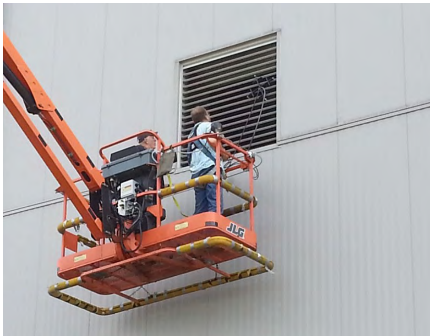
Figure 8. Photo of NIOSH investigator measuring air velocity at an exhaust fan outlet. Photo by NIOSH.
