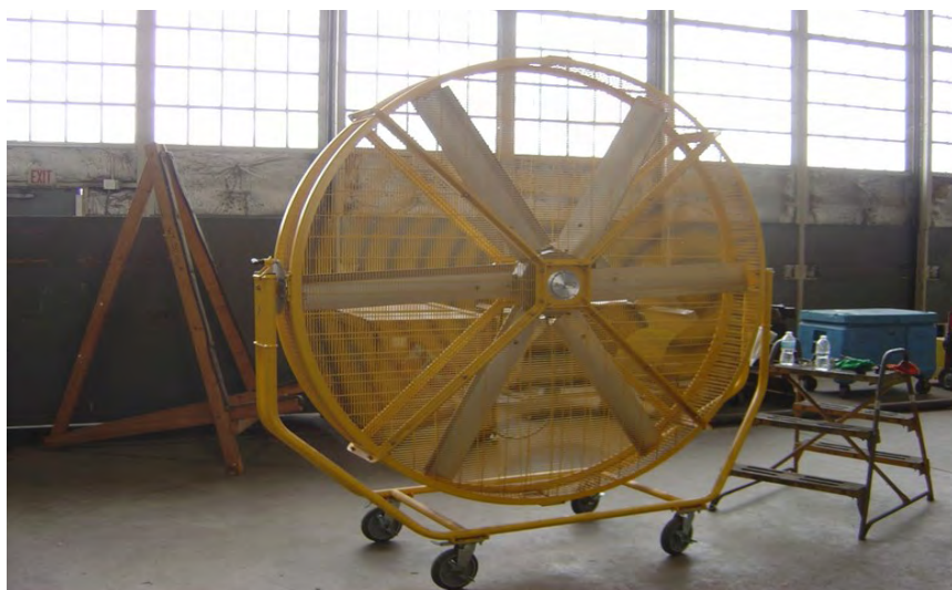
Figure 5. Photo of movable vertical floor fan in a restoration hangar. Photo by NIOSH.
