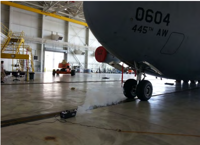
Figure 9. Photo of use of an aerosol-generating smoke machine to visualize airflow patterns near an aircraft. Photo by NIOSH.
