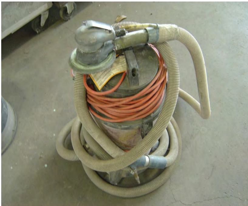
Figure 7. Photo of ventilated hand sander attached to a high efficiency particulate air filtered vacuum. The sander is used by employees in the restoration hangar. Photo by NIOSH.
