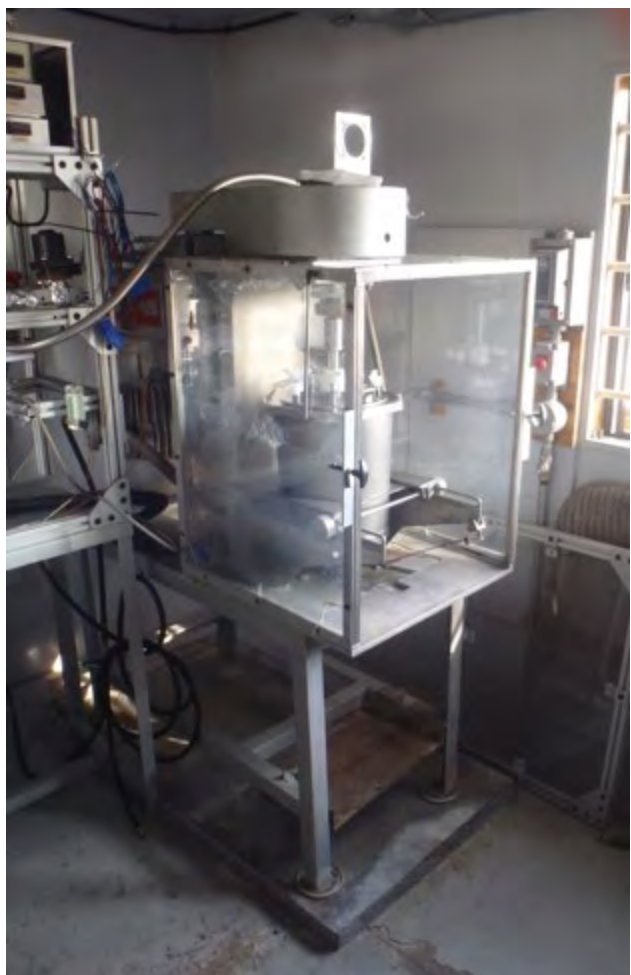
Figure 1. Cryomill inside an enclosure. Photo by NIOSH.
