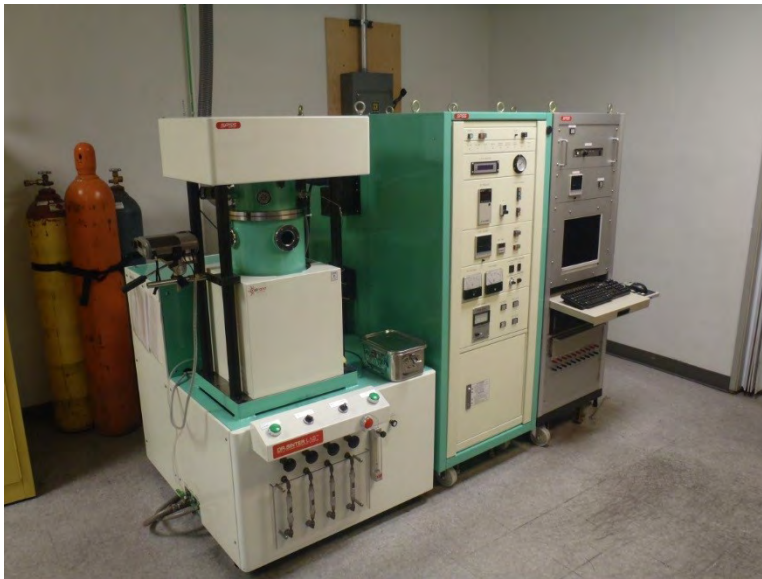
Figure 2. Photo of the SPS machine used for metal powder sintering. Photo by NIOSH.
