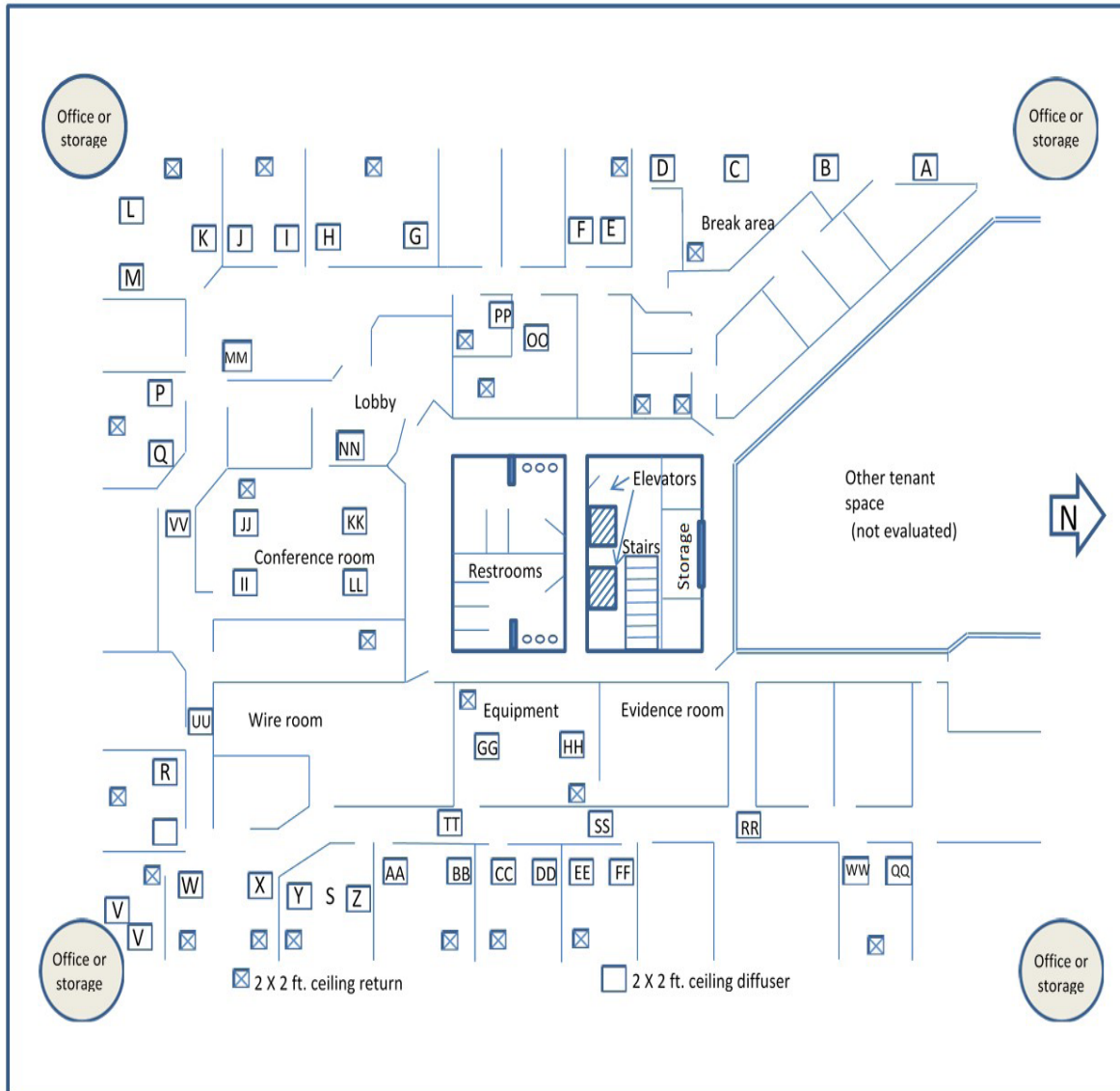
Figure B1. Office diffuser locations, seventh floor
