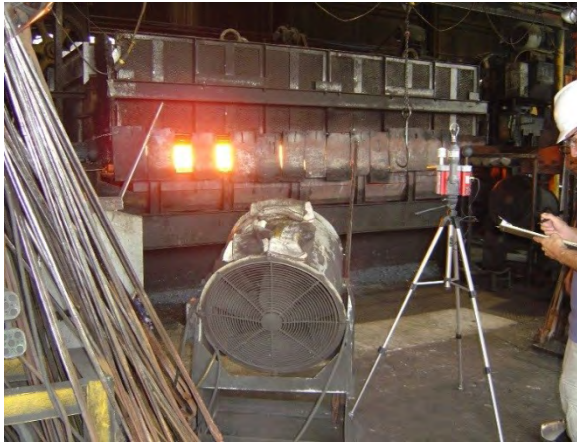
Figure 2. Furnace for heating metal ingots. Small metal flaps hang over the front of the furnace to cover the opening during heating. Photo by NIOSH.
