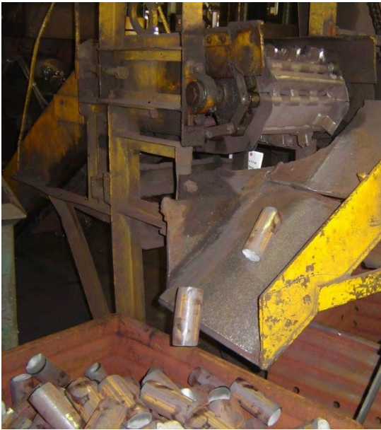
Figure 14. Ingots dropping from the shear onto a metal chute and falling into a metal bin. Photo by NIOSH.
