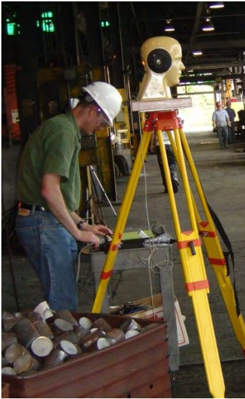
Figure 16. NIOSH researcher preparing to take hearing protector noise attenuation measurements using an acoustic mannequin head. Photo by NIOSH.
