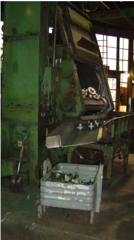
Figure 15. Forgings being dumped from a shotblast onto a vibrating conveyor pan and moving down the conveyor to fall into a metal bin. Photo by NIOSH.
