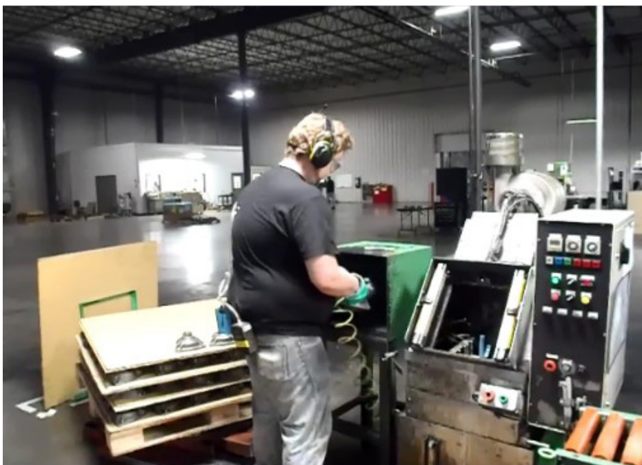
Figure 2. Machine operator standing in front of blow-off box, blowing off finished part before placing it on pallet to his left. Photo by NIOSH.
