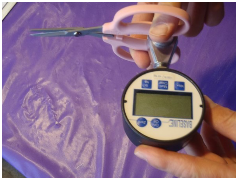
Figure 3. Bud snipping force was estimated by having the employee reproduce the force with the handles of the scissors transmitting the force to the pinch gauge. Photo by NIOSH.
