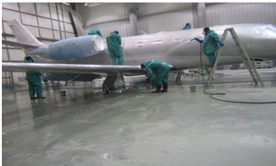
Figure 6. Employees wearing rain suits, full facepiece respirators, rubber boots, and gloves are rinsing an aircraft with water after degreasing inside the stripping bay. Photo by NIOSH.
