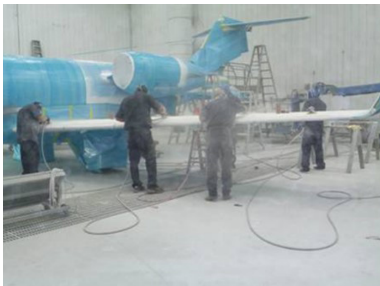
Figure 5. Employees wearing coveralls with hood, goggles, gloves, and full facepiece air purifying respirators while sanding an airplane inside a paint bay with pneumatic sanders that do not have dust control. Photo by NIOSH.
