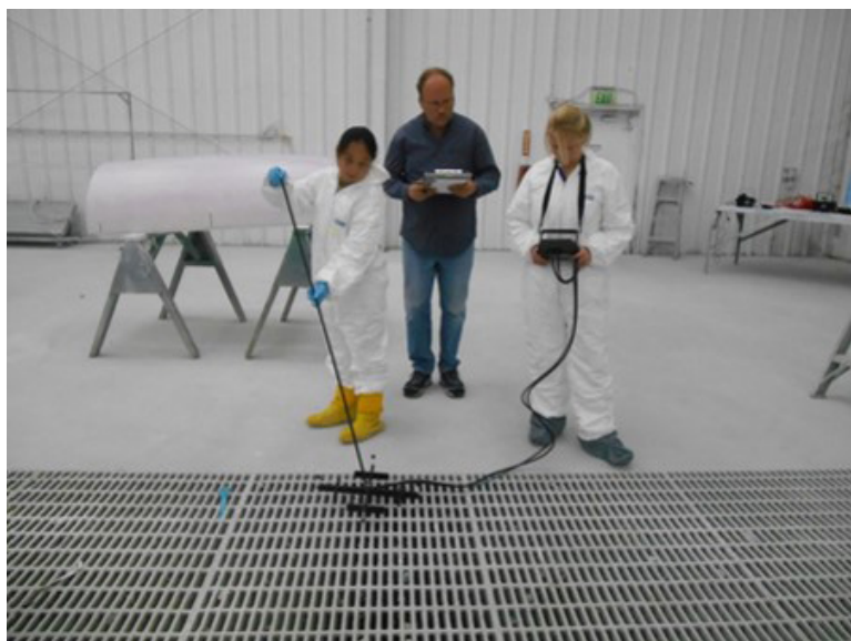
Figure 12. Measuring air velocity and airflow through a paint bay exhaust grates. Photo by NIOSH.
