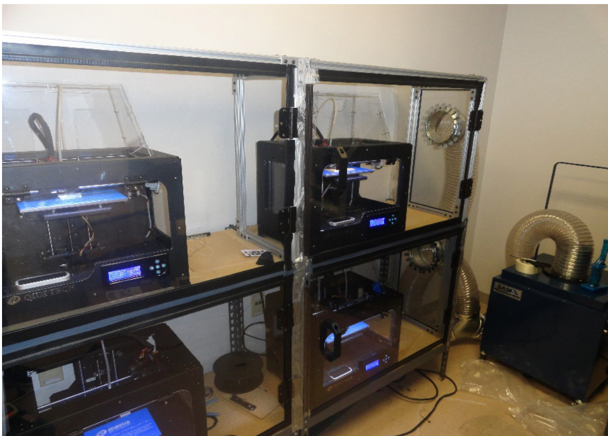
Figure 12. Custom-built ventilated enclosure connected to a floor fan with particle and organic filters. Photo by NIOSH.
