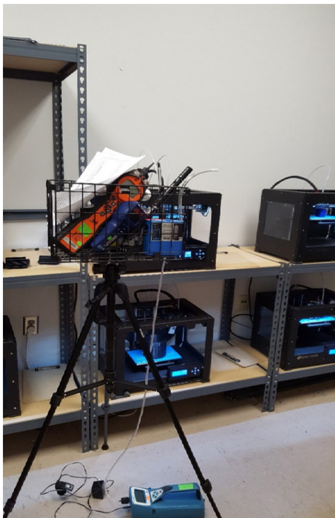
Figure 1. Area sampling station showing real-time monitors and time-integrated samplers in the Print Room. Photo by NIOSH.
