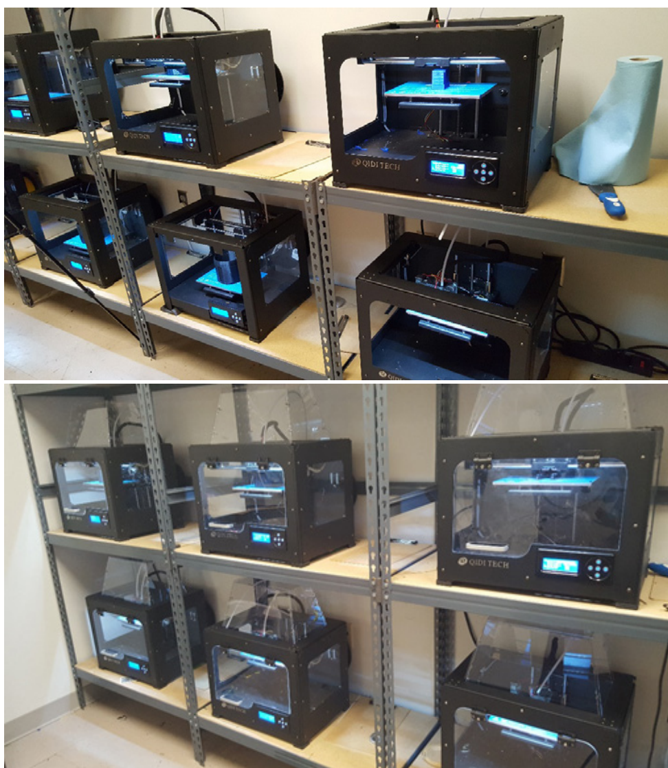
Figure 7. 3-D printers as normally used (top picture) and with the manufacturer-provided plastic covers and doors installed (bottom picture). Photos by NIOSH.
