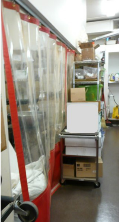
Figure 1. Plastic curtain separating the spice grinding area from the rest of the shop. Photo by NIOSH.
