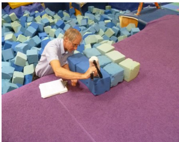
Figure B2. Investigator using a direct reading instrument to measure the bromine content in foam pit blocks. Photo by NIOSH.
