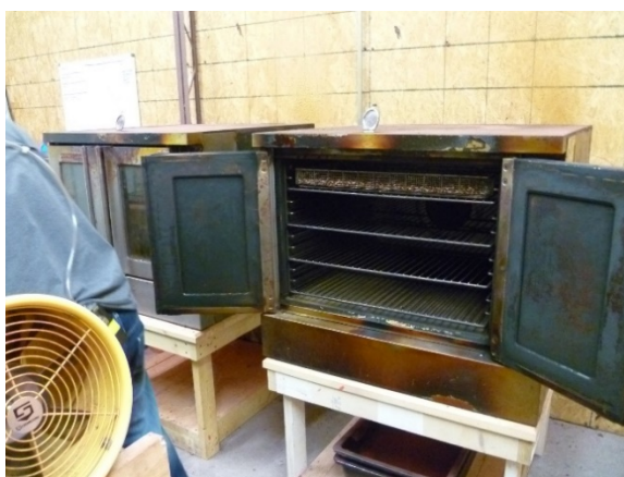
Figure 12. Trays of freshly coated bullets are placed into electrically-heated ovens to harden the paint coating.
