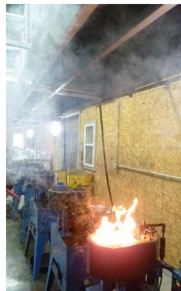
Figure 4. Flux smoke not captured by the overhead local exhaust ventilation.
