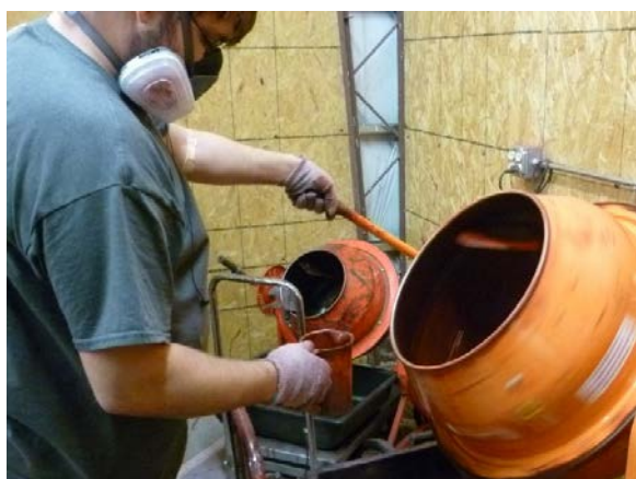
Figure 11. Employee manually pouring a mixture of powdered paint and solvent from a cup into a rotating tumbler containing uncoated bullets.
