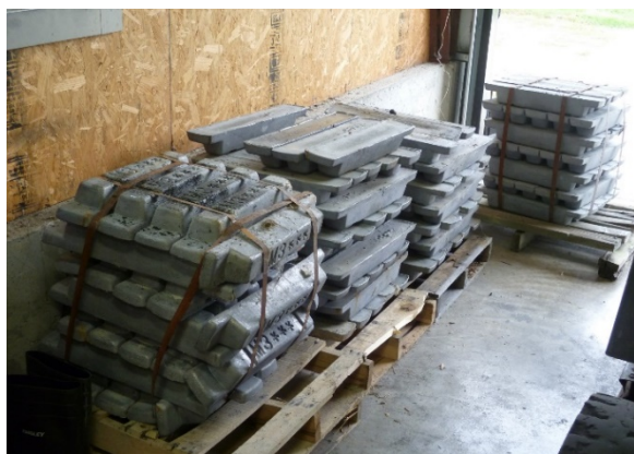
Figure 9. Four pallets of lead ingots (called pigs) stored in the casting bay. Each lead pig weighed about 60 pounds.
