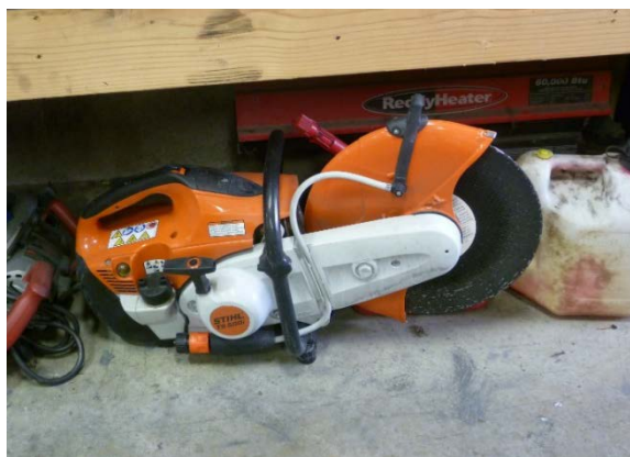
Figure 10. Hand-held, gasoline-powered, water-cooled abrasive cutoff saw. An employee used the saw to cut the 60 pound lead ingots into sizes small enough to fit in the bullet caster melting pot.
