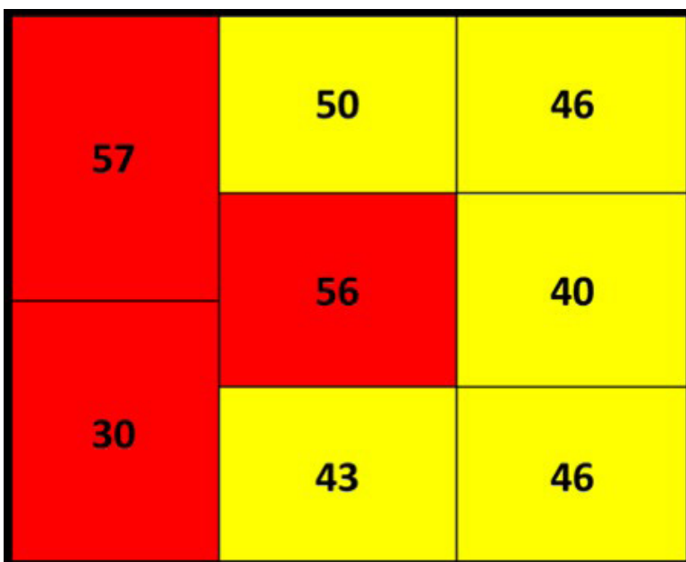
Figure 4. A diagram showing the face velocity measured at different points of the hood. There are only two measurements in the left column because the probe did not fit across the face of the hood three times and needed to be turned to measure the whole face. The red boxes indicate a greater than 20% difference from the average face velocity (46 feet per minute). All measurements were below OSHA and ANSI specifications. Figure by NIOSH.
