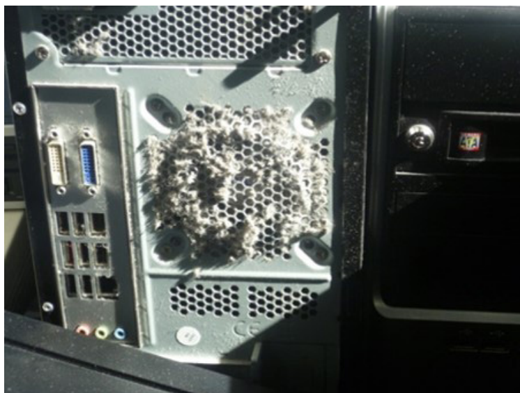
Figure 1. Example of a cooling fan on a piece of electronic equipment that has pulled in a lot of dust from the environment. Photo by NIOSH.
