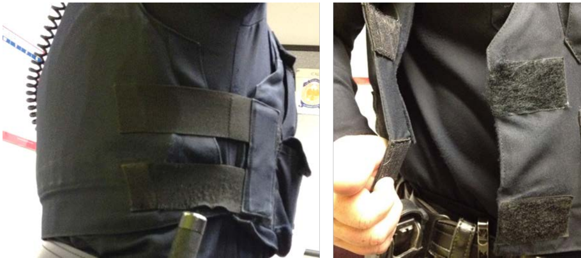
Figure B1. Intact side Velcro closure on external vest (left). Unsecured side of external vest due to worn Velcro pads (right). Photo by NIOSH.
